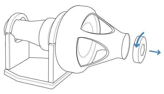
Remove PCMPMIRR mirror array by unscrewing it
